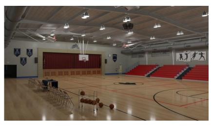
40 - 400W MH lamps16,000W total loadNot dimmable25min warm up time
